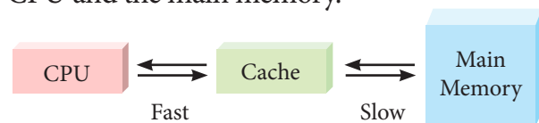
Figure 3.8 Cache Memory Arrangement
