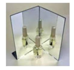
**Figure 6.5** Images formed by inclined mirrors
