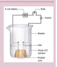
of a 6V battery through a bulb and a switch as shown in Figure. Now pour some dilute HCl in the beaker and switch on the current. Repeat the activity with dilute sulphuric acid, glucose and alcohol solutions. What do you observe now? Does the bulb glow in all cases?
