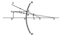
**Figure 6.10** Image formation in a convex mirror
