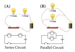
Figure 4.11 Series and parallel connections
