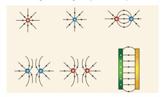
Figure 4.2 Electric lines of force
