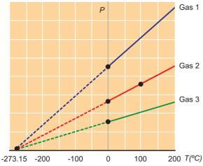
**Figure 7.7** Variation of pressure (P) with temperature (T).
