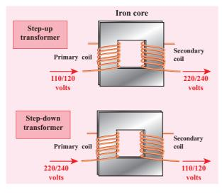
Figure 5.20 Step up and step down transformers
