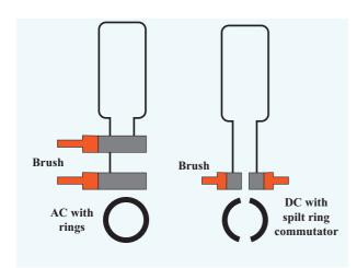
**Figure 5.19** Comparison of AC and DC generators
