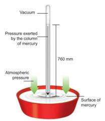
Figure 3.6 Mercury barometer
