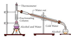
Figure 10.9 Fractional distillation
