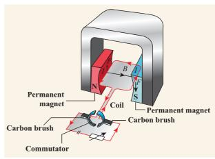
Figure 5.13 Principle of electric motor
