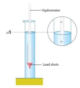
Figure 3.10 Hydrometer
