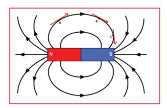
Figure 5.2 Magnetic field lines
