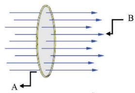
Figure 5.3 Magnetic flux
