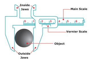
Figure 1.2 Vernier Caliper
