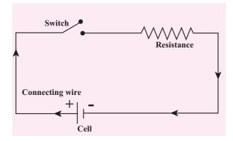
Figure 4.10 Typical electric circuit
