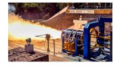
✓ Skyroot Aerospace recently conducted a successful test-fire of the Kalam-250 at ISRO's Satish Dhawan Space Centre. This second stage of the Vikram-1 space launch vehicle features a carbon composite rocket motor, EPDM thermal protection, and precision thrust vector control. Developed by Skyroot Aerospace, it will propel the launch vehicle from the atmosphere into outer space, playing a vital role in its ascent.
