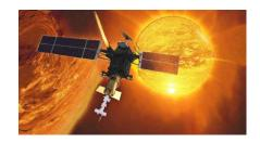
✓ The Plasma Analyser Package for Aditya (PAPA) payload on the Aditya-L1 satellite detected the impact of coronal mass ejections (CMEs) on solar wind. The PAPA payload is an energy and mass analyzer that measures solar wind electrons and ions. It contains two sensors, the Solar Wind Electron Energy Probe (SWEEP) and the Solar Wind Ion Composition Analyser (SWICAR).
