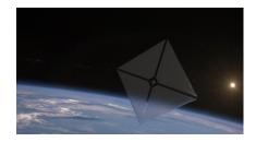
✓ NASA recently launched a space mission from New Zealand, deploying the Advanced Composite Solar Sail System spacecraft aboard Rocket Lab's Electron rocket. The spacecraft utilizes solar energy for propulsion, orbiting 1,000 kilometers above Earth with an 80 square meter sail. Key objectives include demonstrating solar sail effectiveness and maneuverability.
