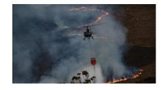
✓ The Indian Air Force deployed MI 17 V5 helicopters equipped with Bambi Buckets to combat forest fires in Nainital. The Bambi Bucket, also known as a helicopter bucket, is a specialized firefighting tool used since the 1980s. It's suspended under the chopper and filled from rivers or ponds, releasing water via a pilot-controlled valve. Its features include quick filling, storage within the helicopter, and precise water discharge, aiding in combating inaccessible wildfires.
